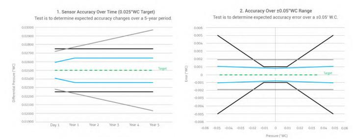
Sensor A: 18.8% Rdg. Error; Sensor B: 10.0% Rdg. Error; Setra 5.7% Rdg. Error
