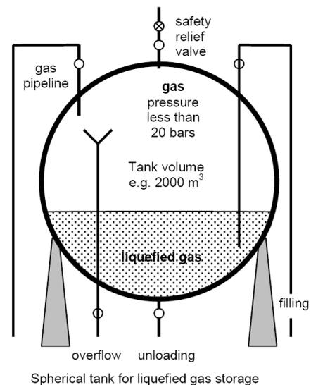
Pressure tanks are equipped with a fill level indicator with alarm facilities and sensors to measure the interior temperature continuously to switch on a cooling sprinkler system in case of temperature alarm.
