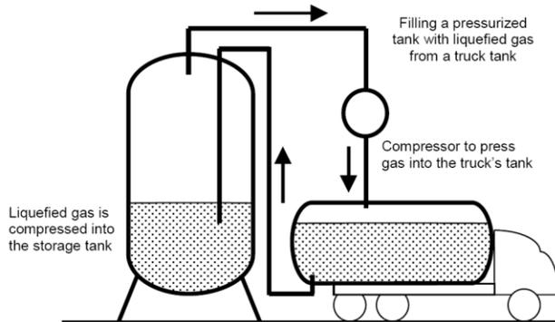
Tank filling is made by two connecting tubes, one for the gas, one for the liquid. The gas is drawn out from the storage tank and by means of a compressor it is pressed into the truck's tank. The resulting pressure forces the liquefied gas into the storage tank then. This is a more or less dangerous process, especially when making the necessary tube connections. Gas leaks can occur and gas detection is recommended. The most famous gases kept in a pressure tank are ammonia, chlorine and LPG.
