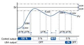
▲ LBA operation stop by PV entering LB,DB range ▼ LBA operation stop if control output is not 0% or 100%
