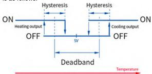
Figure 24. Heating & Cooling Hysteresis
