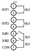
Figure 13. PD520 & PD530 Relay Connections
