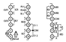
Figure 6. PD510 Connector Diagram
