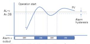
Figure 28. High Absolute Alarm Operation
