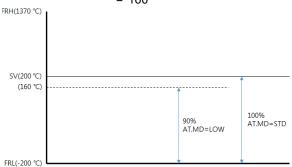
Figure 33. Standard and Low PV Auto-Tuning SV
