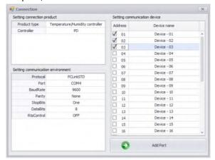
Note that for USB connections, it may be required to check what virtual com port is being used for the USB connection in the computer's Device Manager tool.
