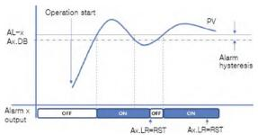
Figure 31. High Absolute Alarm with Latch Function
