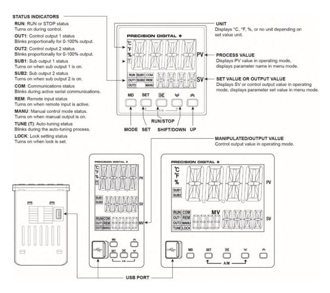
Figure 22. Front Panel Buttons and Indicators
