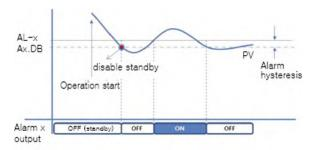
Figure 30. High Absolute Alarm Operation with Standby
