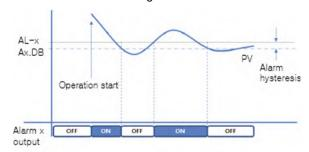
Figure 29. High Absolute Alarm Operation without Standby
