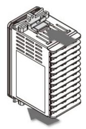
Figure 3. PD520 and PD530 Mounting Bracket Installation
