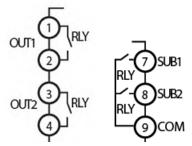
Figure 12. PD510 Relay Connections
