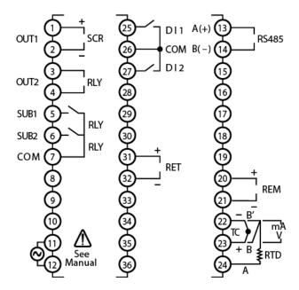
Figure 7. PD520 & PD530 Connector Diagram
