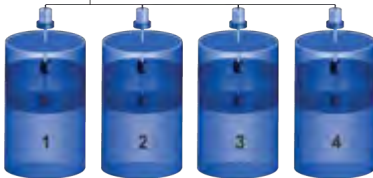
Tanks with Multivariable Level Transmitters
