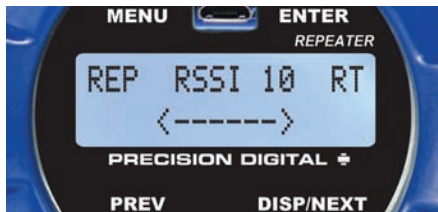
▲ Close-up of PDW30-RNA Repeater Display
