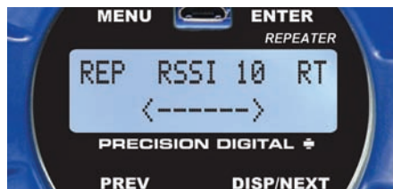
▲ Close-up of PDW30-RNA Repeater Display
