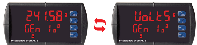
Upper line toggles between 241.58 and Volts and the lower line displays Gen 1
