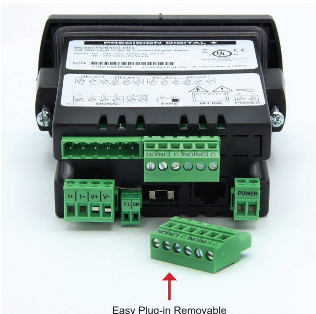
Easy Plug-in Removable Terminal Connectors
