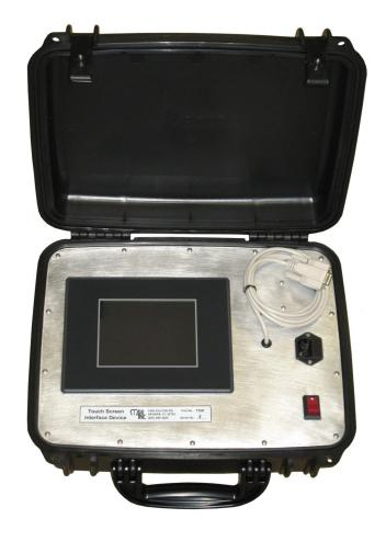
The Touch Screen Interface Device (TSID) consists of a 6 inch Touch Screen panel made by Automation Direct, housed in a durable carrying case with a power cord and an interface cable for connection to the serial port. It is programmed as a Modbus Master that continually polls the device it's connected to.
