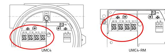
Output Signals shown in Ex-ia type of protection
