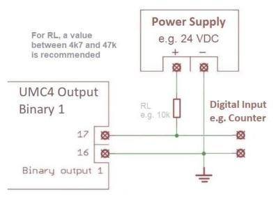
Image 3: Example for wiring a Binary output
