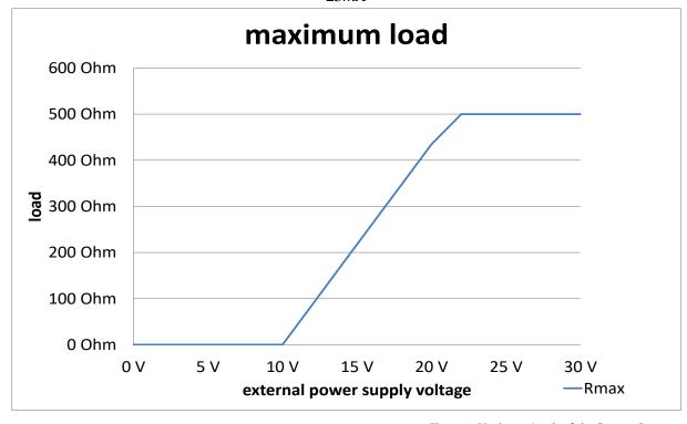
Figure 1: Maximum Loads of the Current Outputs
