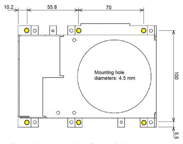
**Note:** The above depiction is not in scale and is therefore not suitable to be used as a mounting template.
