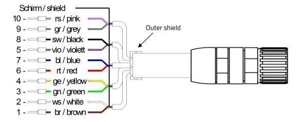
The outer shield is connected to the terminal box cable gland at one end, and the connector's outer-case at the other end. The inner shields of the wire-pairs are connected to each other (drilled together) and connected to the "Schirm / Shield" terminal in the junction box.
