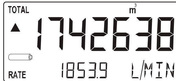
Fig. 4: Example of low-battery alarm
