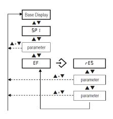
By pressing  $\blacktriangle + \blacktriangledown$  simultaneously the menu will return to the base display or automatically after ca. 60 s without operation.
