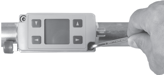
Fig. 8 Tighten mounting screws
