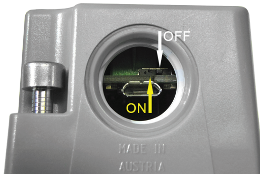
Fig. 11 Bus termination resistor
