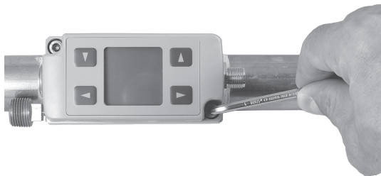
Fig. 20 Unscrew mounting screws
