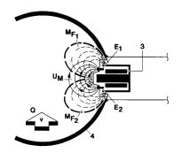
MF1, MF2: Magnetic Field E1, E2: Electrodes
