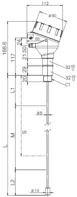
Single Rod Probe, PTFE Coated Flange Disk
