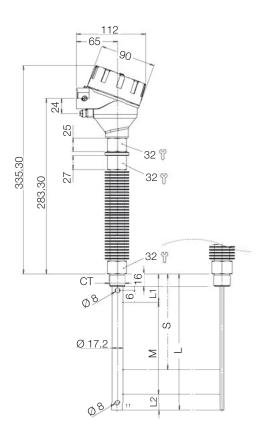
NGM Assembled in a Bypass Tube: Option "...B"
