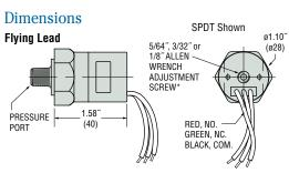
\* Adjustment screw is located under protective screw.
