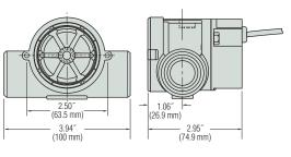
High Resolution Black Rotor PPS composite. Each of the six rotor arms is magnetized. A PTFE loaded bushing ensures long life.
