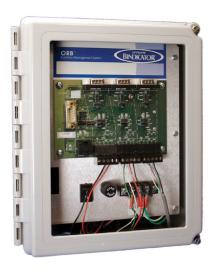
The ORB<sup>™</sup> is a controller that connects to process instrumentation via serial and 4-20 dedicated interfaces. The  $ORB^{^{\intercal M}}$  contains a database and integrated web server. It becomes a gateway between process instruments and the Internet. The ORB™ web pages can be accessed using any browser from any device that has Internet connectivity.
