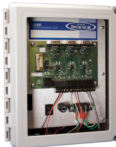
The ORB™ is a controller that connects to process instrumentation via serial and 4-20 dedicated interfaces. The ORB™ contains a database and integrated web server. It becomes a gateway between process instruments and the Internet. The ORB™ web pages can be accessed using any browser from any device that has Internet connectivity.
