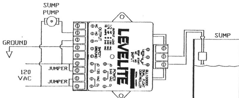
EXAMPLE OF SUMP-PUMP WIRING
