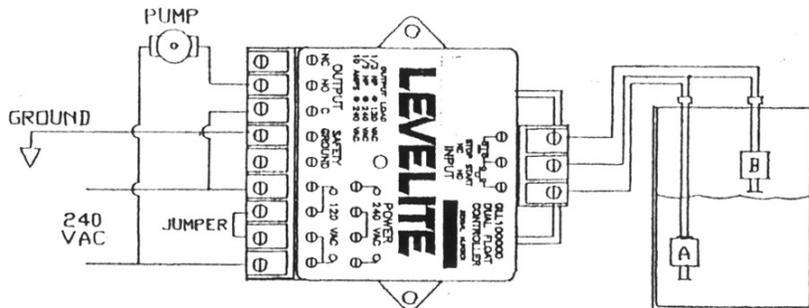
EXAMPLE OF AUTOMATIC FILL WIRING.
