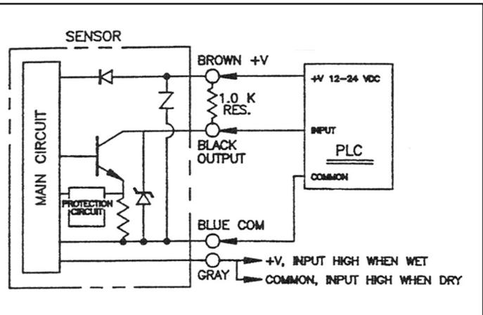
Note: Common wire (gray) must be connected to common (-) or V+(+) supply of power supply.
