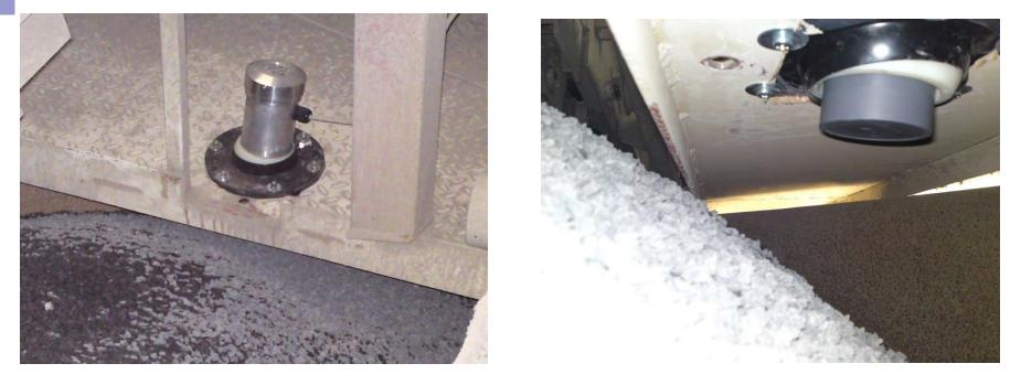
**Application Problem**: Plastic pellets with dust, very steep angle of repose.
