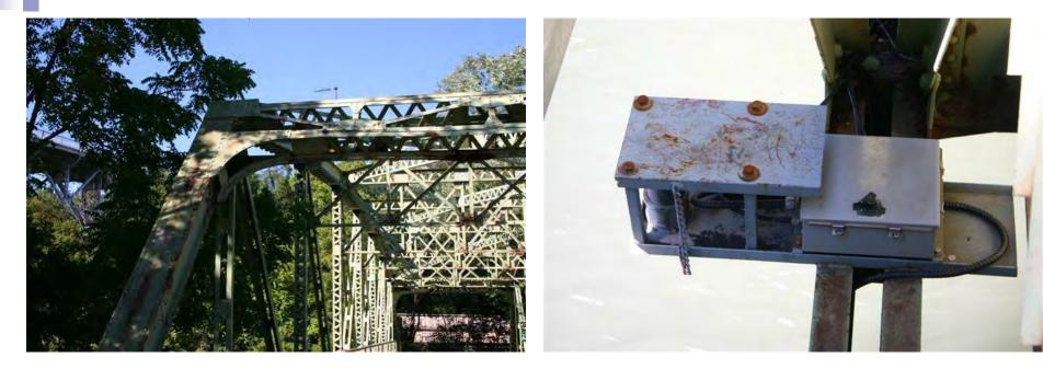
**Application Problem**: Extremely low power consumption, battery supply with RF transmitter of the current output 4mA to 20mA.
